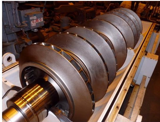
Figure 30: Compressor Rotor with Electroless Nickel Coating
