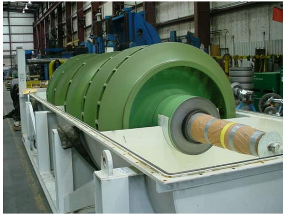
Figure 29: Compressor Rotor with a PTFE Topcoat
