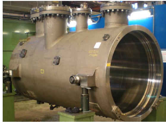
Figure 7. LP compressor casing before hydraulic test
